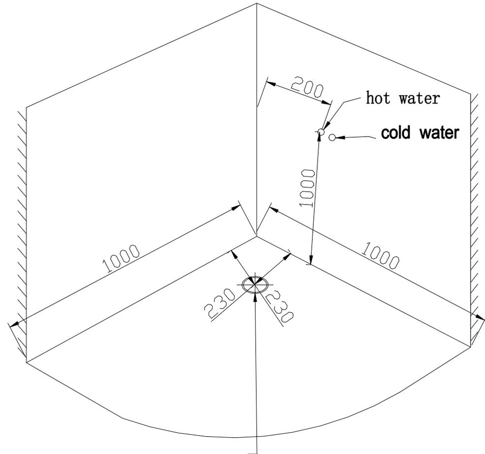
drain hole can not small than 50mm
